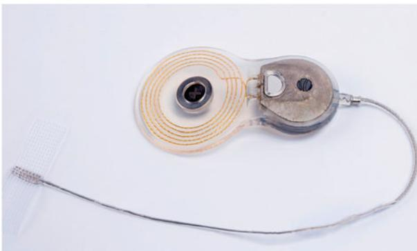
**Figure 1.** Photograph of Nurotron auditory brainstem implant device.
