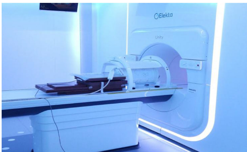
Figure 3 MAMA phantom. The "Maternal Anthropomorphic Analogue" (MAMA) validation phantom, consisting of an Arc-CheckMR and solid water, shown on the Elekta Unity couch.
